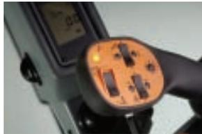
By the touch of a button on the ergonomic multifunction handle, the unloading auger is extended and engaged.
