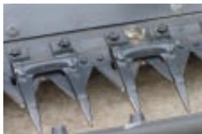
Optional SCH cutterbar knives on the 8200 bolt to the bar in alternating pattern to cut on both the top and bottom, vastly increasing cutting efficiency and extending wear life.
