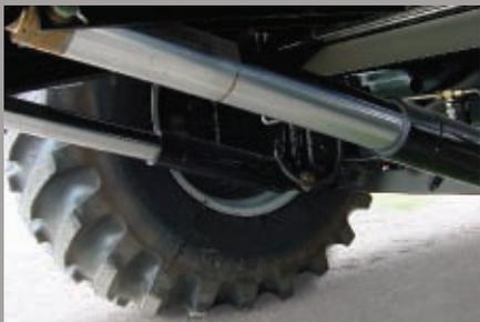
Two 3 $\frac{1}{2}$ -in. (89 mm) header lift cylinders are capable of lifting all GLEANER headers.
