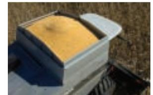
Engineers designed the grain tank for natural grain flow, drawn off by a single auger in the bottom of the tank.
