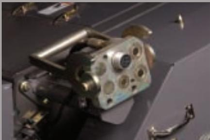
All header wiring and hydraulic couplers are now unified in a single multicoupler for easy, error-free, one-point connection.
