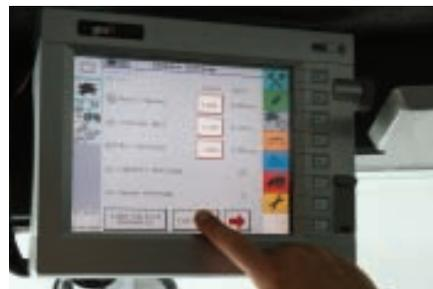
Monitored by in-cab digital readout, fan speed can be adjusted from the operator's console via electric linear actuator for maximum performance and productivity (A85).
