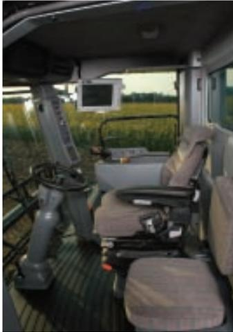
The air-ride seat automatically provides infinite weight adjustment, ergonomic fitting, adjustable arm rests and cushion angle, integrated backrest extension, adjustable lumbar support, seat belt and more.
