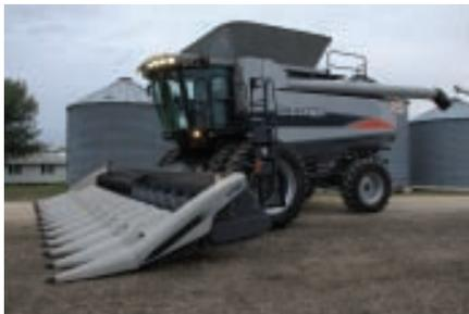
Wide platforms on the rear of the combine allow for easy access to the grain tank for inspection. Steps and platforms in the grain tank facilitate service.
