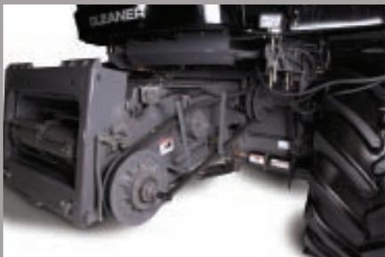
A variable-speed corn header drive allows the operator to change the corn header and feed chains' speed to adapt to crop changes for the best productivity.
