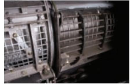
The high-wire concave, unique to all GLEANER R5s, brings 1.4 in. (35 mm)-spaced wires closer to the threshing surface for complete, gentle threshing. Front grate adjusts independently of the concave assembly for varying conditions.
