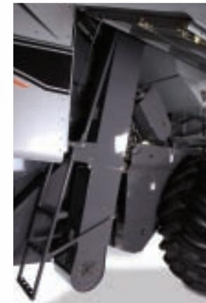
A large-capacity clean-grain elevator moves the grain to the grain tank. Easy to service with the bottom adjustment.
