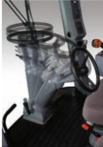
The leather wrapped steering wheel allows multiple tilt and telescopic positions to fit the operator and large footrests for added comfort.
