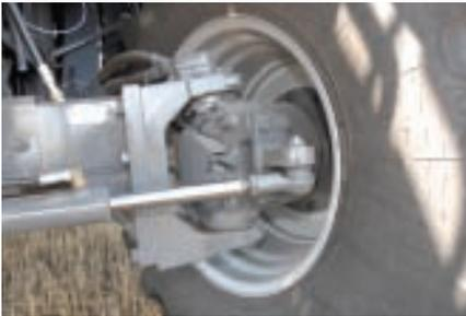
Pressure-sensitive cam lobe RWA motors engage easily as hydrostatic pressure increases. No mechanical lock-in or lock-out required. Two-speed drive motors are used on the A85 model.
