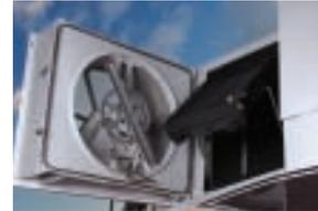
A rotary screen, which is hydraulically driven for improved reliability, ensures constant and even airflow to the cooling system. The screen and cooler both swing out of the way for easy and quick cleaning.
