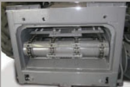
Two undershot four-strand feed chains provide high capacity and reliability. (Compression springs maintain feed chain tension.)
