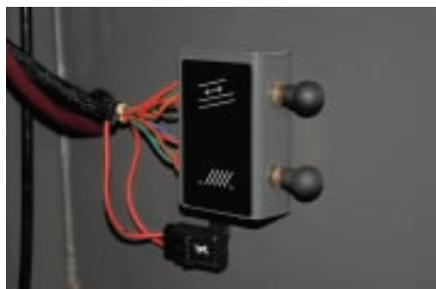
Sieve and chaffer electric adjustment control is available on the side of the combine or in the cab using the Console II (A85).
