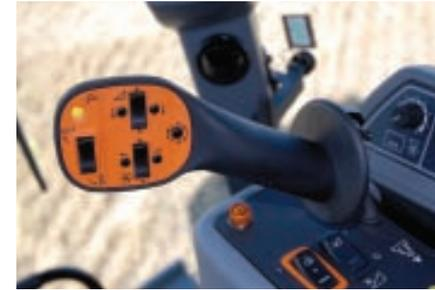
The unloading auger's electro-hydraulic swing control operates conveniently from the main hydro handle. A choice of automatic or manual auger engagement lets you unload automatically without distraction while maintaining the ability to top off a cart from the operator's seat.
