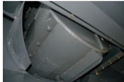
The A5 rotor's patented direct discharge throws material directly out of the thresher, eliminating the need for discharge beaters. The simple but advanced design prevents unnecessary straw damage, as well as eliminating horsepower-robbing drives, shafts and belts.
