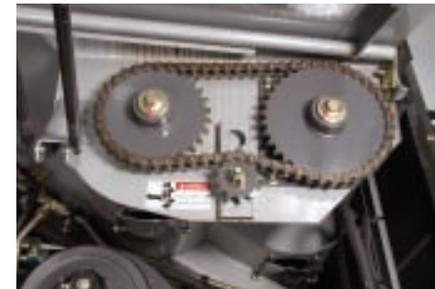
Two bearing-supported axles drive the unloader augers using strong gears for added life. Wide openings for inspection and cleaning, plus exterior-located grease zerks, make service simple and quick.
