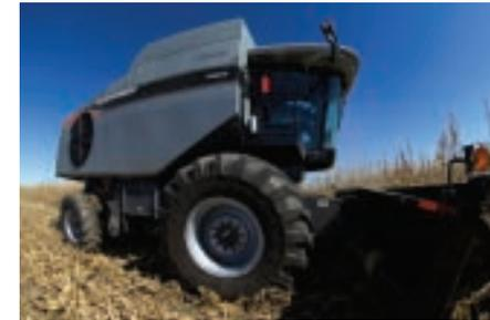
Drive and steering tires in a variety of sizes, plies and ratings, including optional Michelin MegaXbib® low-pressure, steel-belted radials, designed to spread a 19% greater footprint than competitive radials, providing greater flotation and reducing compaction.
