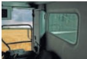
A clear view through the rear cab window, combined with mirror-handy perforated portholes on both upper corners of the grain tank remove any mystery about grain level.
