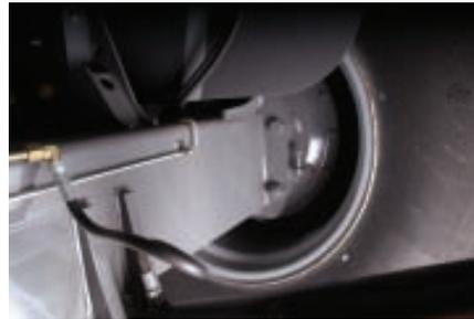
Heavy final drives offer a 7.066-to-1 gear reduction for transmitting tractive force to the ground without limiting single or dual wheel options.
