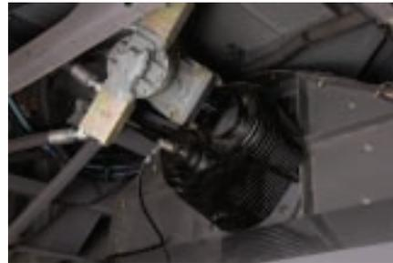
The rotor is powered by a hydrostatic system fully regulated by electronic control of oil flow and rotor speed. A three-speed heavy-duty planetary gearbox drives the rotor on the A85.
