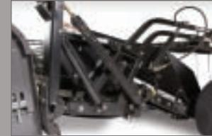
GLEANER Ultra-Float Suspension uses a heavy spring and shock system to dampen rugged terrain and smooth out the rough spots. An advanced, hydraulically positioned windguard, which can be raised or lowered from the cab, improves feeding and reduces crop rolling.
