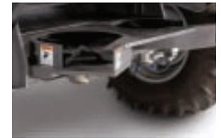
For extra heavy chaff spreading, add the optional hydraulic chaff spreader. Two hydraulically driven impellers promise extra-wide distribution.
