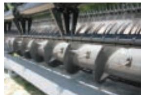
Full-fingered auger with 7-in. (178 mm) flighting ensures a smooth, even flow of crop material to the feed chain system.
