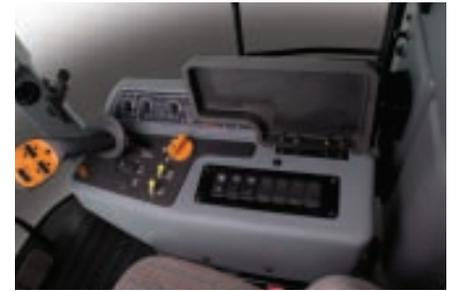
One button varies rotor speed via an electro-hydraulic valve. Concave settings are also adjustable to changing crop conditions, all from the operator's seat.
