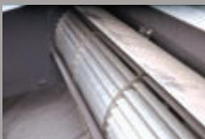
A high-volume, low-pressure curtain of air provided by the 1,150 rpm transverse-flow fan blows away light chaff as the accelerated grain passes through unaffected.
