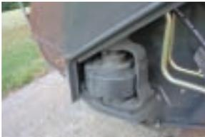
Hydraulically driven SCH planetary gear sickle drive system moves the sickle at 1200 strokes/min with a 3 1/8-in. (80 mm) stroke for smooth cutting and increased performance.
