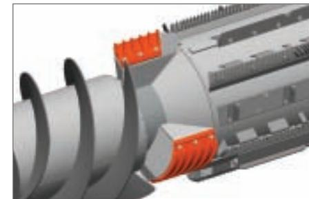
The patented intake uses edge-hardened flights to feed crop into the threshing system positively yet nonaggressively. Material moves efficiently with minimal damage to grain.
