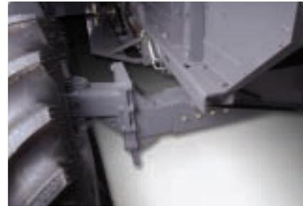
Adjustable steering axle goes from 119 in. (3.0 m) to 144 in. (3.66 m) in 6-in. (152 mm) increments. The A5 Series axle also allows adjustment of axle height by 4 in. (100 mm) to adapt to different tire sizes.
