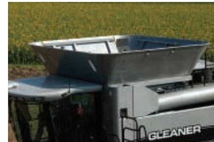
Quick-release grain tank extensions fold down easily, reducing the transport and storage height to 144 in. (3.65 m)\* for the A65/A75 and 147 in. (3.73 m) for the A85, respectively.
