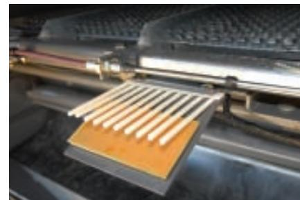
Grain loss sensors keep track and alert the operator.
