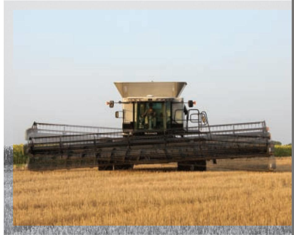
As an option to the GLEANER header control system, the SmartTrac lateral tilt mechanism (LTM) can be used to manually or automatically follow every contour of the field with any of the 3000, 7200 or 8200 Series headers.
